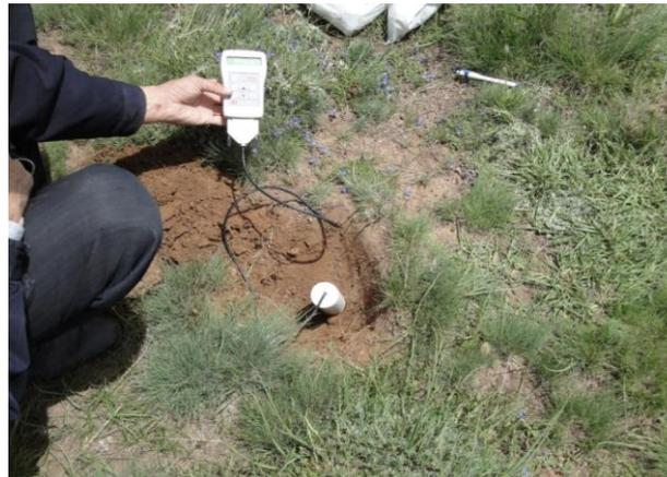
Fig. 2. Soil moisture monitoring by using a Delta-T Devices Ltd version 4.0 type HH2 Cambridge-England
