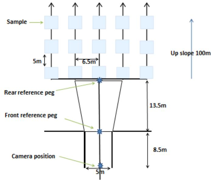
Fig. 3. The Monitoring Site Layout
